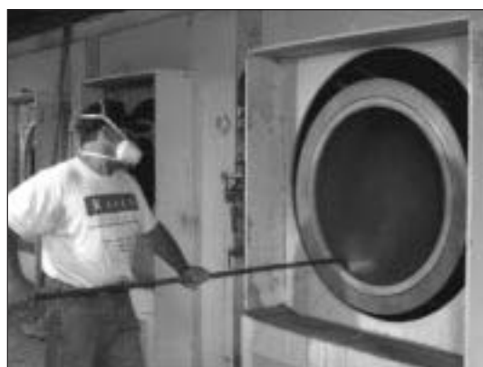
Each layer of glass and resin is rolled to remove air bubbles and to insure a dense uniform laminate.
