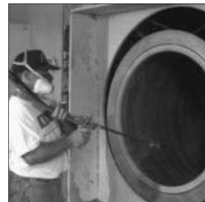
Polyester resin is sprayed onto the mat while the mold cylinder is revolving. This centrifugal action forces the resin through the mat, saturating it.
